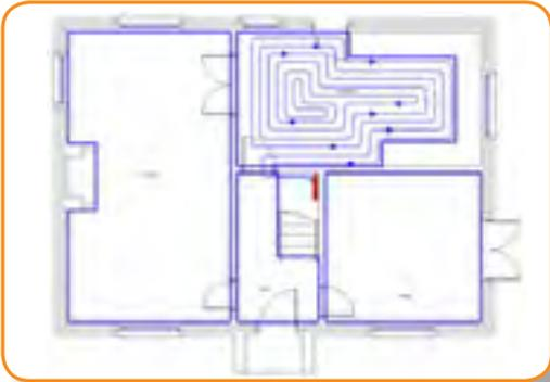
**STEP 3.** To complete the loop, return pipe inside the existing pattern back to the manifold maintaining the pipe spacing (typically 200mm).
