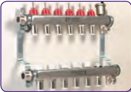
**STEP 1.** Fix the pre-assembled manifold to the wall, allowing enough height to accommodate the insulation and screed depth and also the pipe work and conduit elbows.
