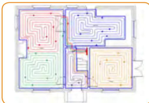
**STEP 6.** Continue the process for the remaining rooms, ensuring pipes are not crossed in the floor.
