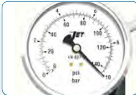
**STEP 5.** If all is well, increase the pressure to 10 bar and leave for a further 10 minutes while checking for leaks or pressure drops.
