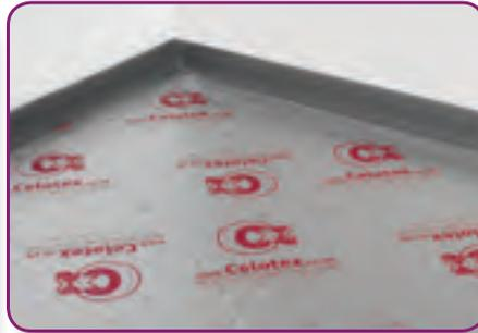
**STEP 2.** Floor panels should be fitted to a suitable flat sub base. Extra insulation maybe required to match design or building regulations and to ensure that any downward heat loss does not exceed 10 Watts m<sup>2</sup> in accordance with BSEN1264.
