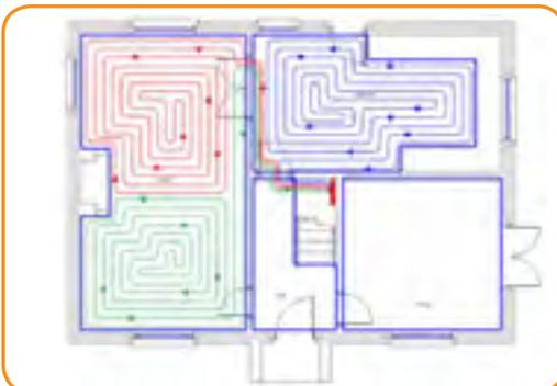
**STEP 5.** In rooms with more than one circuit care should be taken to ensure enough room is left for flow and return runs back to the manifold.
