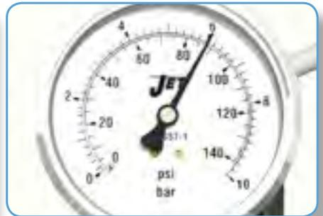
**STEP 6.** If all remains well, reduce pressure to operating pressure. For screeded floors, pipework should be left to approximately 3-6 bar until the screed has been laid and dried to protect pipework from damage. Consult screed supplier for drying out and curing time.
