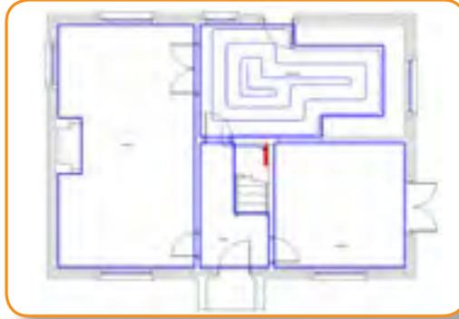
**STEP 2.** Working from left to right or right to left, install first loop working into the centre of the room.
