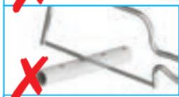
Don't use hacksaws to cut the pipe or leave burrs on the end of the pipe.
