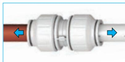
Pull to check connection is secure. It is good practice to test the system prior to leaving the site or before use. Our recommended test procedure is shown in our Technical Checklist.
