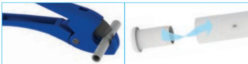
Ensure the pipe is free of score marks. Cut the pipe square. When using Speedfit Barrier Pipe cut along an insertion mark. We recommend the use of JG Pipe Cutters.
