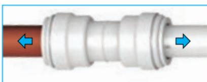
Pull to check the connection is secure. It is good practice to test the system prior to leaving the site or before use.
