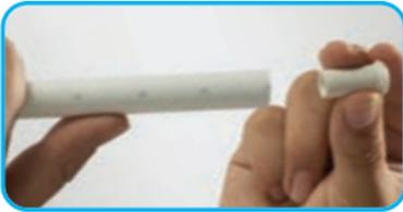
This makes the pipe completely round ensuring the best possible seal between the 'O' ring and the outside diameter of the pipe. When using Speedfit Pipe with a compression fitting the Insert gives rigidity to ensure the pipe does not collapse under pressure as the compression olive is tightened.
