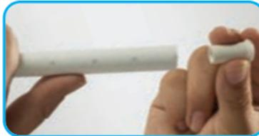
This makes the pipe completely round ensuring the best possible seal between the 'O' ring and the outside diameter of the pipe. When using Speedfit Pipe with a compression fitting
