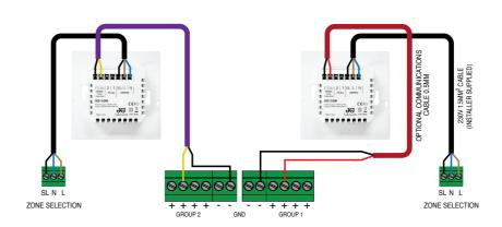
Please Note: If the Hot Water Timer is part of a group then the communication connection must be connected to Group 1.
