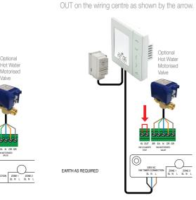
Option 2 - Connect Cylinder Thermostat directly to
