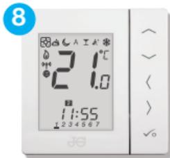
Thermostat returns to home screen. **Testing:** Set to call for heat. Check TRV's are opening and Boiler Receiver is receiving the signal. Turn down the thermostat and check TRV's shut and boiler receiver turns off.
