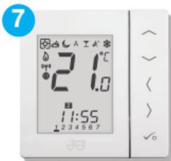
Thermostat returns to home screen. **Testing:** Set thermostat to high temperature and wait for a call for heat. Check the Wireless Boiler Receiver is receiving the signal and switching on and off.
