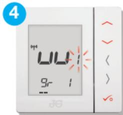
**UU** icon flashing to request the number of the Wiring Centre you wish to pair with (see Identifying Wiring Centre - page 9). Use **^** and **v** to select the required number. Press **CONFIRM** ✓
