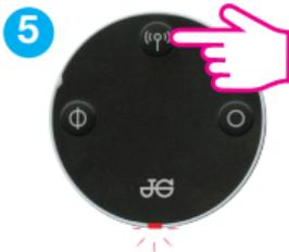
Press Pairing Button on TRV(s) for 10 seconds until pairing light on the TRV starts to flash. Maximum of 6 TRV's can be paired at the same time.
