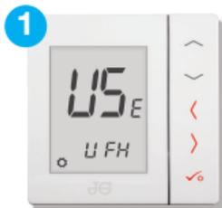
Start up screen as shown. Hold bottom 3 buttons to scroll to screen **2**.
