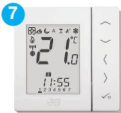
Thermostat returns to home screen. **Testing:** Set thermostat to high temperature and wait for a call for heat. Check the Receiver is receiving the signal and switching on and off. If there is also a boiler receiver fitted to the network check that this is responding.
