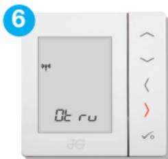
Next press > arrow on thermostat to start pairing process. **Do not** press Confirm ✓ as it will abort the pairing process and user will have to start again.
