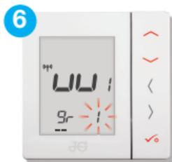
6 Zone number flashing. Using the
