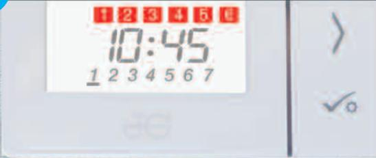
The **PROGRAM INDICATOR** runs on a **24-HOUR** cycle. It has the option of up to six programmable periods running over a 24 hour cycle.
