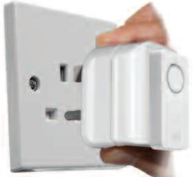
**4** Insert the adaptor into 230v mains outlet.
