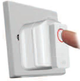
**8** When all devices are paired, press and hold the button for 5 seconds. The button will stop flashing, indicating that the network is closed to new devices.
