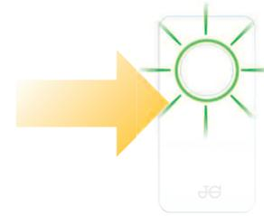
**i** To exit identify mode, press for 1 second. Alternatively, identify mode will automatically time-out after 10 minutes
