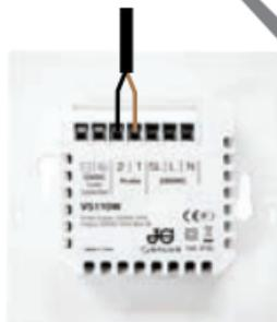
HW Timer connected to cylinder thermostat.
