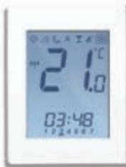
Use the up arrow to select the frost protection temperature.
