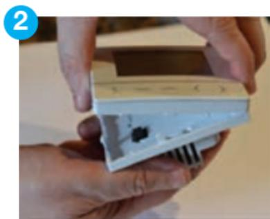
Carefully remove the front housing.
